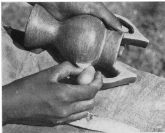
FIG. 25. Catawba potter using a polishing stone. Note bone scraper lying beneath right hand.
